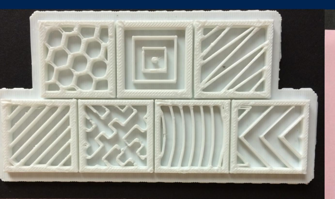
Top to bottom, left to right: Honeycomb, Concentric, Line, Rectilinear, Hilbert Curve, Archimedean Chords, Octogram Spiral
